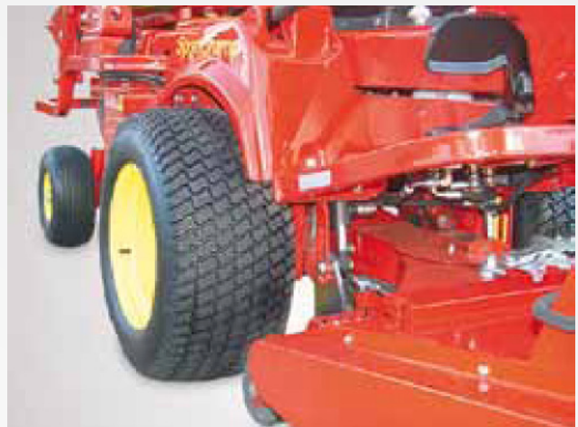
Tires specially for use on grassy surfaces ensure low pressure on the ground
