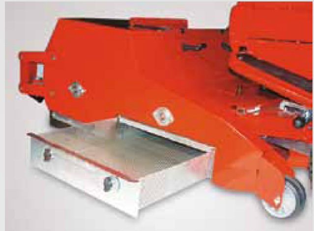
The vibrating screen separates dirt from the infill and spreads the infill on the artificial turf again at the same time
