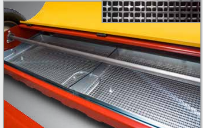
Vibrating screen continuously adjustable from 4 - 10 mm
