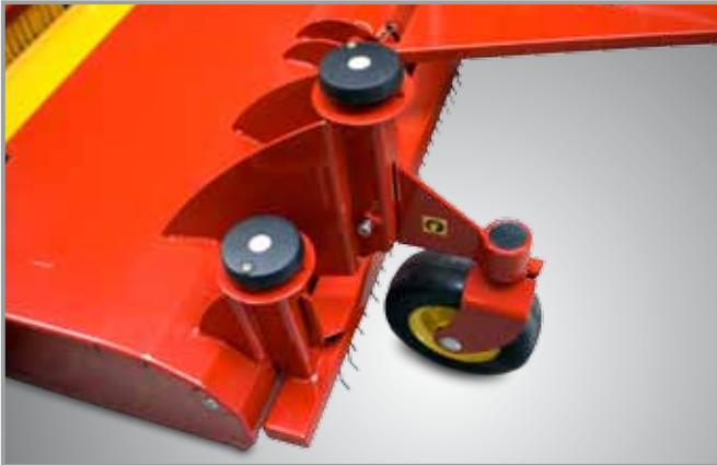
Adjusting spindles for working depth and tow bar
